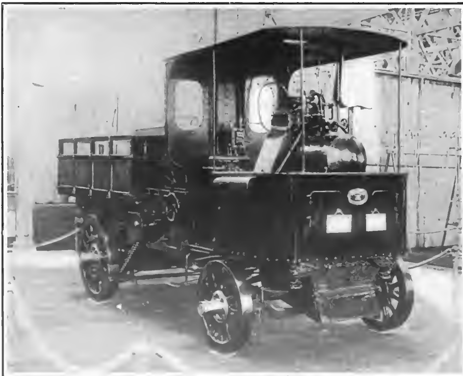
TURGAN-FOY STEAM TRUCK—ONLY HEAVY COMMERCIAL VEHICLE IN FRENCH SECTION.
